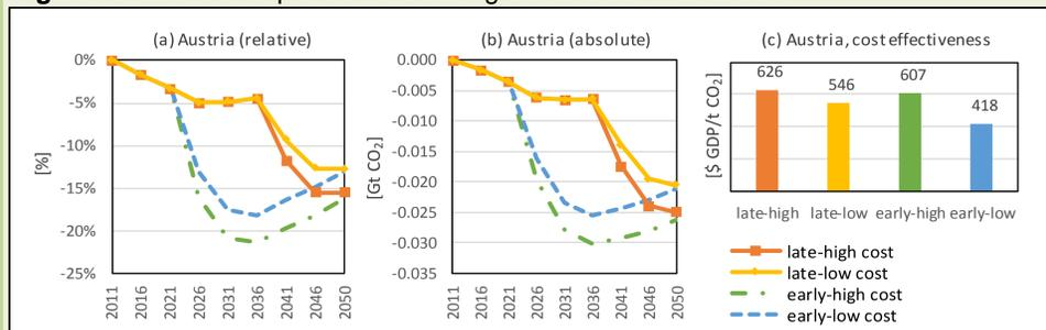
**Figure:** Changes in CO2 emissions (a-b) and cost effectiveness (c) by an EU-wide transition to climate neutral electricity and iron and steel production (all changes relative to Baseline).
